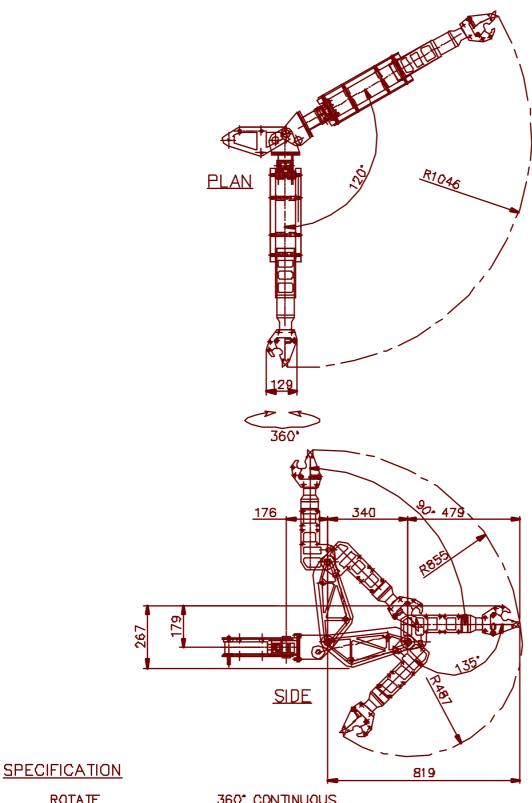
ROTATE TORQUE AT 140 BAR LIFT AT 140 BAR 360° CONTINUOUS 38 Nm
